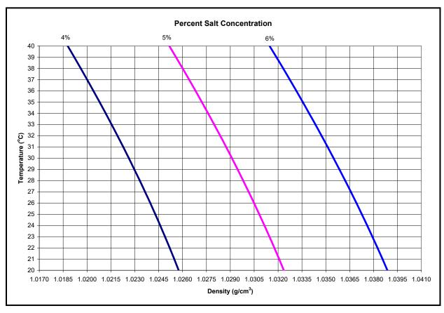
Figure 509.7-3. Variations of density of salt (NaCl) solution with temperature.<sup>1</sup>
