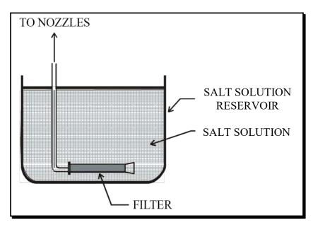
Figure 509.7-1. Location of salt solution filter.
