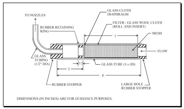
Figure 509.7-2. Salt solution filter.
